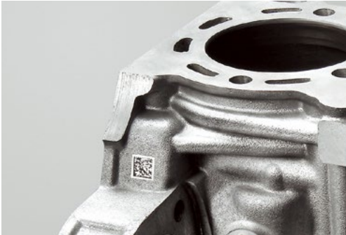
White + Black-oxidized marking: Aluminum casting
